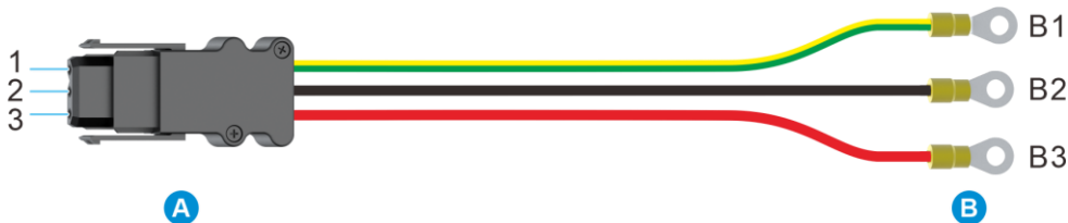
Figure 10-4 -48V DC Power Cable
