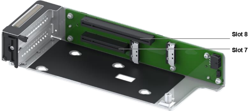
Figure 6-4 RC5306N2B Riser Card Installed in I/O Module 3
