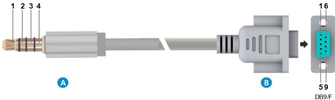
End A of a serial cable is a 3.5 mm audio plug, and end B is a 9-pin D-shape molded plug. Both end A and end B are numbered as pin numbers.
