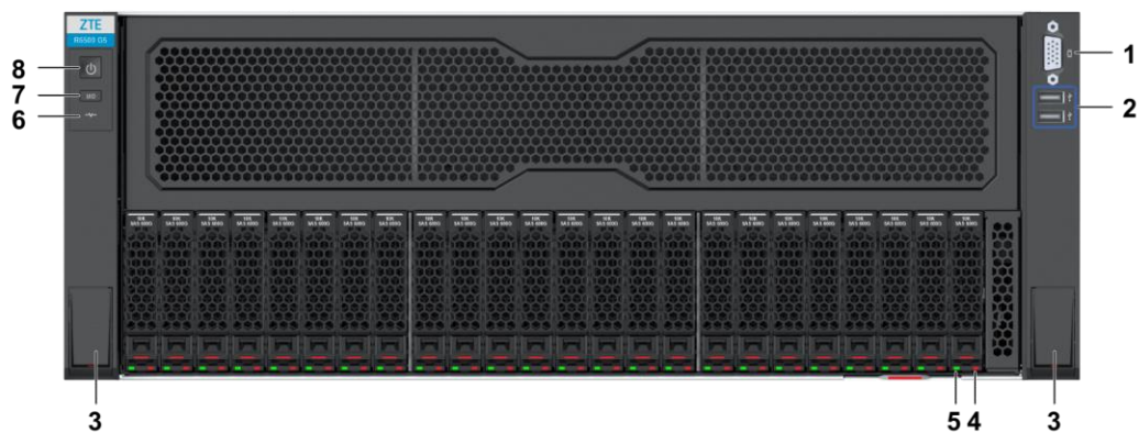
Figure 2-4 Front Panel with Twenty-Four Vertical Disk Slots
