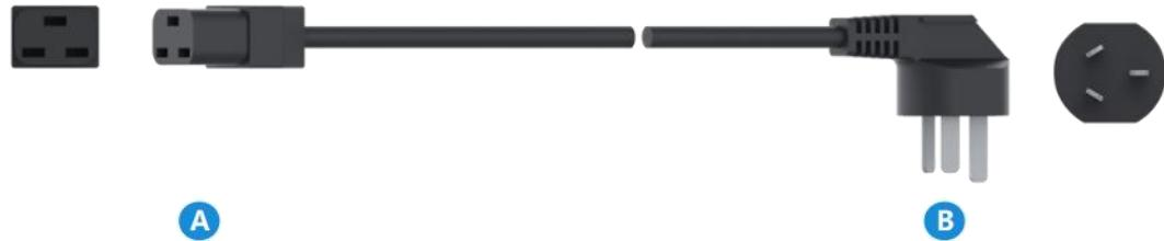
End A of the power cable is a C19 female connector, and end B is a 16 A three-flat-pin male plug. The power cable is a black power cable.
